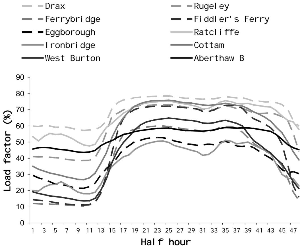
**Figure 2. Spread of load factors for independent and integrated generating plants**
